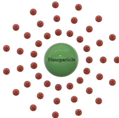
Fig 2. Charging Salt ions bind to nanoparticle [Varanasi et. al unpublished]
